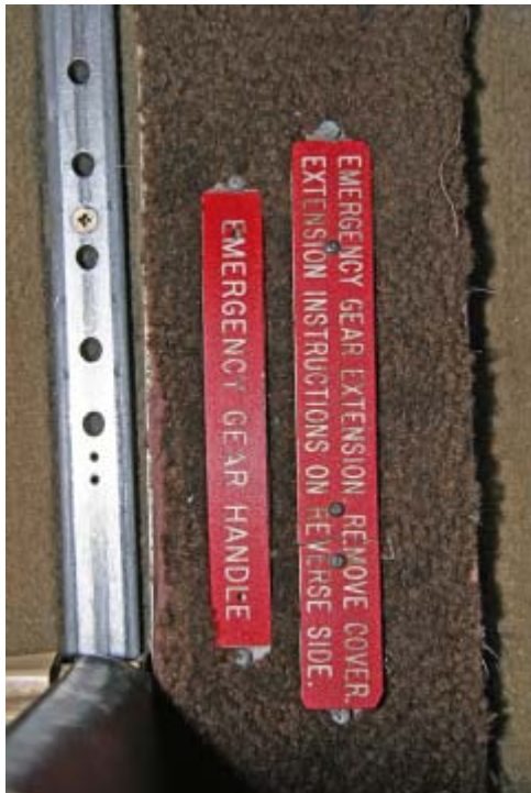
Figure 9, Cover Plate, Emergency Gear, front side
