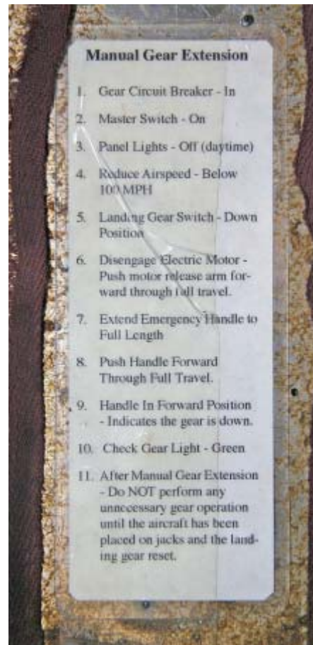
Figure 10, Cover Plate, Emergency Gear, back side
